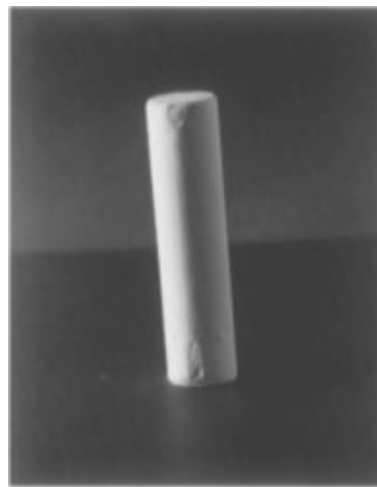
Figure 2. Photograph of a monolithic silica aerogel (1 cm × 3.2 cm) prepared by polymerizing tetramethoxysilane (TMOS) in supercritical carbon dioxide (SCCD).
